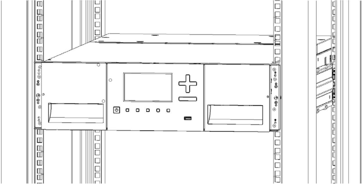
8. Use a Phillips screwdriver to tighten the screws on each side of the module.
