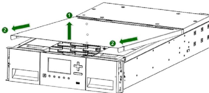
2. Install top cover on the Expansion Module that will be installed on the top of the library.
