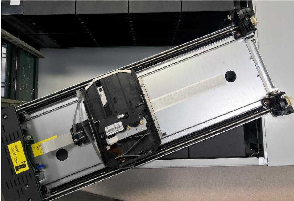
5. On the top of the robotic assembly where the spooling cable is attached, use a small flat head or Torx screwdriver driver to press and push the small latch that unlocks the spooling cable.
