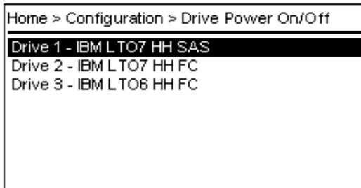
1. The page provides a list of all installed drives. Select the drive that you want to power on or off and press **Enter**
