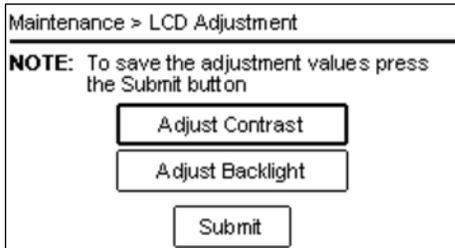
2. The **Adjust Contrast** button is active. Press **Enter** to open the contrast adjustment screen.
