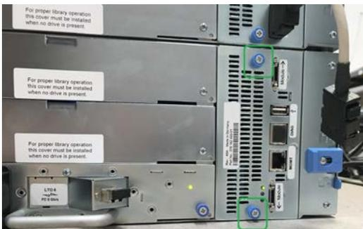
2. Using the thumbscrews, slowly remove the library/expansion controller from the module.
