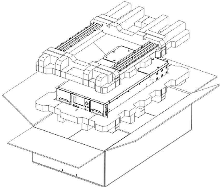
4. Make sure the box is aligned properly before opening the box. The arrows on the box should be pointing upwards.
