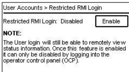
2. Press **Enter** to enable the Restricted RMI Login. The following screen will be shown to inform the user that the Restricted RMI Login is enabled.
