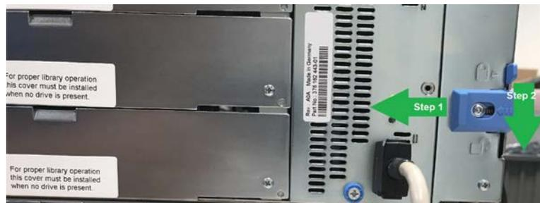
5. Disconnect and completely remove the expansion interconnect cables from the Base Module and from the adjacent modules. Removing the expansion interconnect cables completely prevents damaging the cables when moving the module in and out of the rack.
