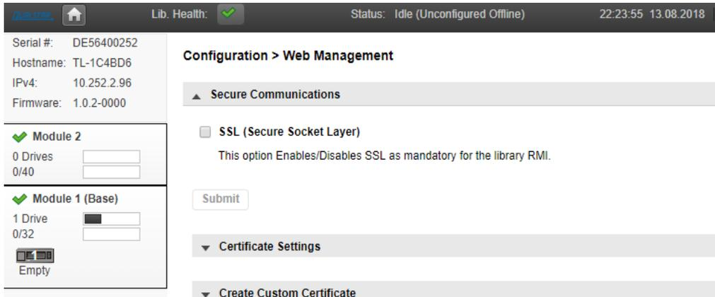
To enable/disable SSL, select the checkbox next to SSL.
