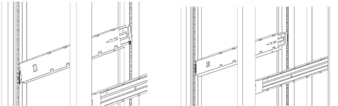
6. Place the library at the front of the rack on the support angles of the sliding rails and push it into the rack to the back stop.
