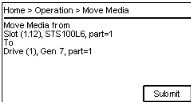
4. Pressing the **Enter** button submits the move command and starts the Move Media operation. Once the command is finished the page will be switched back to the first page. Pressing the **Back** button shall abort the procedure and take the screen back to the Operation menu. Using the left and right buttons on the OCP panel will allow the user to step through the pages again and change the selection.
