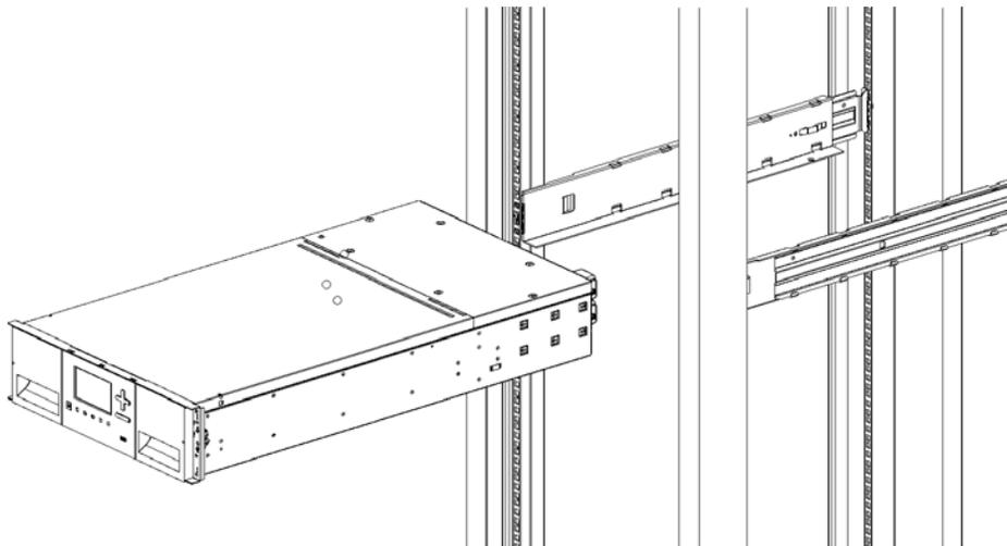
7. If you are installing multiple modules, verify that this module has been installed directly above or below its adjacent module and is contained within the correct 3U volume. The gap between modules must be less than 4 mm.
