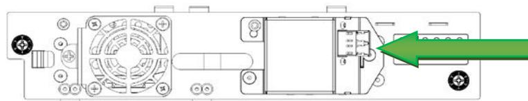
2. Attach the other end of the FC cable to a switch or HBA.
