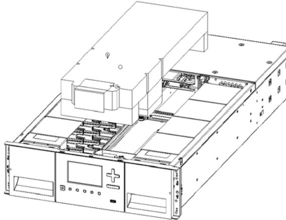
12. If you are installing a Base Module only without an Expansion Module install the top cover again on the Base Module
