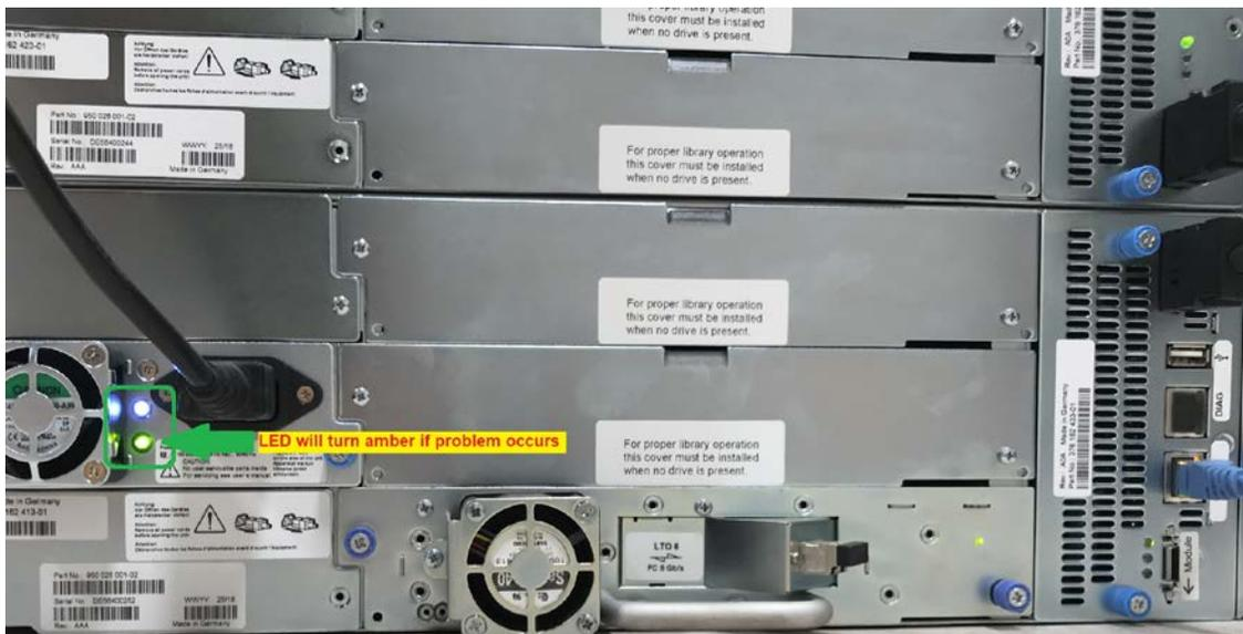
2. Unplug the AC power cord from the power supply you are replacing.
