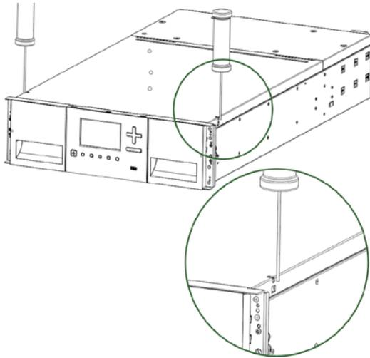
10. Lift the cover front end and pull gently forward to disengage from the pivot point at the unit center
