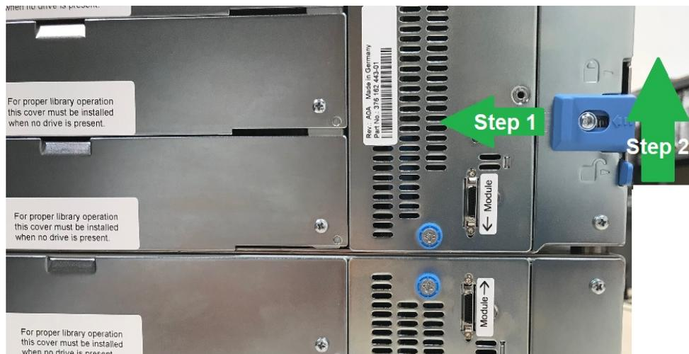
3. Verify that the lowest module in the library has its alignment mechanism in the unlocked position
