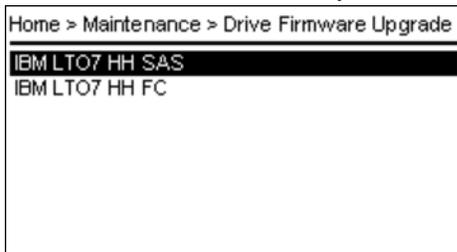
To update the drive firmware from the OCP, the drive firmware files needs to be available on a USB drive.
