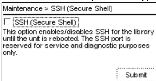
1. Press **Enter** to check SSH (Secure Shell) check box. Now **Submit** is activated.
