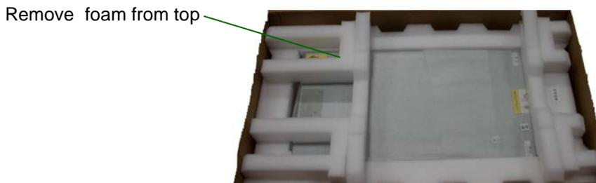
With assistance, lift the module out of the bottom foam nest, remove the wrapping from the module and then place the module on the work surface.
