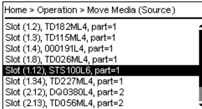
2. Pressing the **Enter** button opens the destination screen. A list will be shown like below. Pressing the **Back** button will take the screen back to the Operation menu. Navigate with the **Up** or **Down** buttons to select the destination element.
