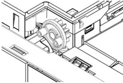
7. Push the robotic assembly down slowly until the platform of the robotic assembly is approximately 10 cm (4 inch) lower than the top of the module.
