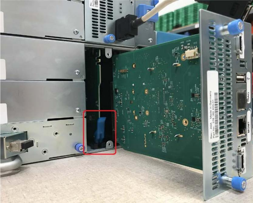
4. Slowly slide out the Drive Power board out of the module.
