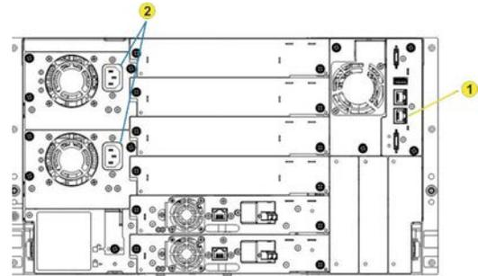
**4** For remote access, connect an **Ethernet cable** from the bottom Ethernet port on the library module controller to your network.
