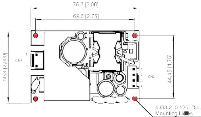
Figure 4-2 ML100 Mounting Hole Locations
