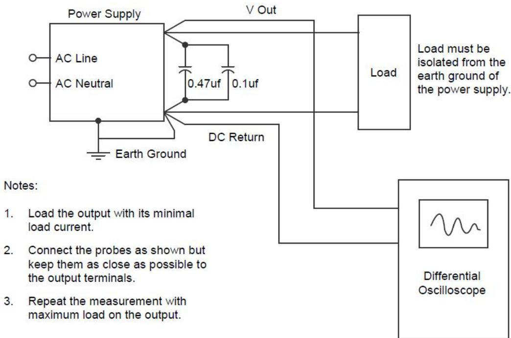
**Note:** The ML100-12 and -15 are measured with 10µf. The ML100-24, -28 and -36 are measured with 1µf. The ML100-48 is measured with 0.1µf. Do not parallel with 0.47µf.
