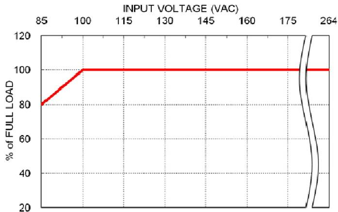
**Figure 3-2 Load vs. Input Voltage: ML100 Series**
