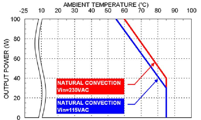
Derating Curve vs. Ambient Temperature
